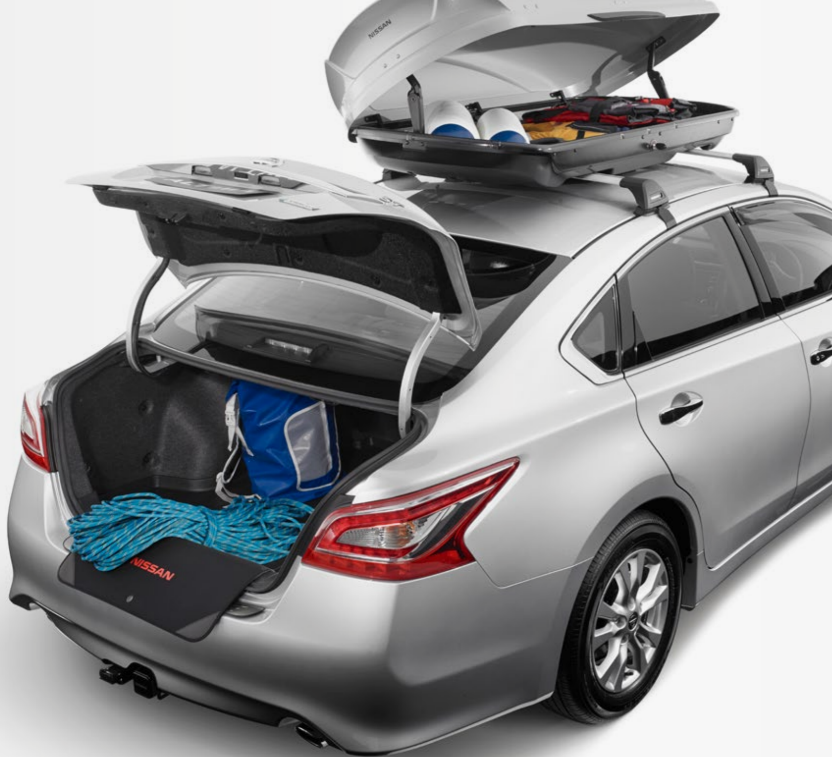
Rear Protection Tray Easy to clean and protects the cargo floor area from dirt and spillages
